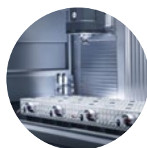
Fixed table with hydraulic connections.
