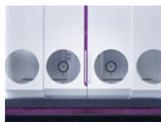
Totally encapsulated working area and safety windows. (Standard).
