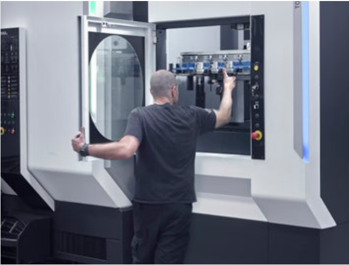
This new ATC system design increases the productivity and machine efficiency allowing risk-free changes outside the working area, loading / unloading the magazine while the machine is running and an easy access to the machine all maintenance elements.
