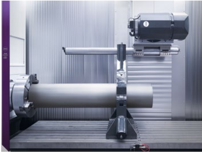
These extraordinarily rigid long boring bars give the machine the capacity to perform internal turning operations.
