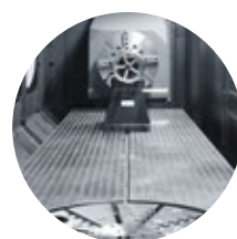
Threaded fixed table for no magnetic materials.
