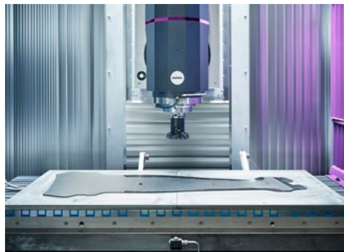
Customize the fixed table with magnetic clamping systems for a direct positioning of parts and/or devices.
