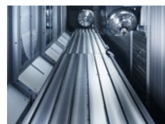
Up to 12.000 mm long working fixed table with "T" slots. (Standard).
