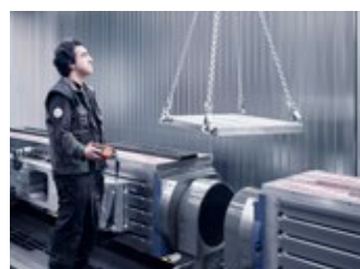
Standard convertible roof for an easy loading/unloading of parts by crane. (Standard).
