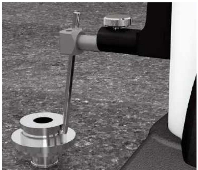
Determination of the height of a groove on a piece integrated in a measuring device for endoscopy
