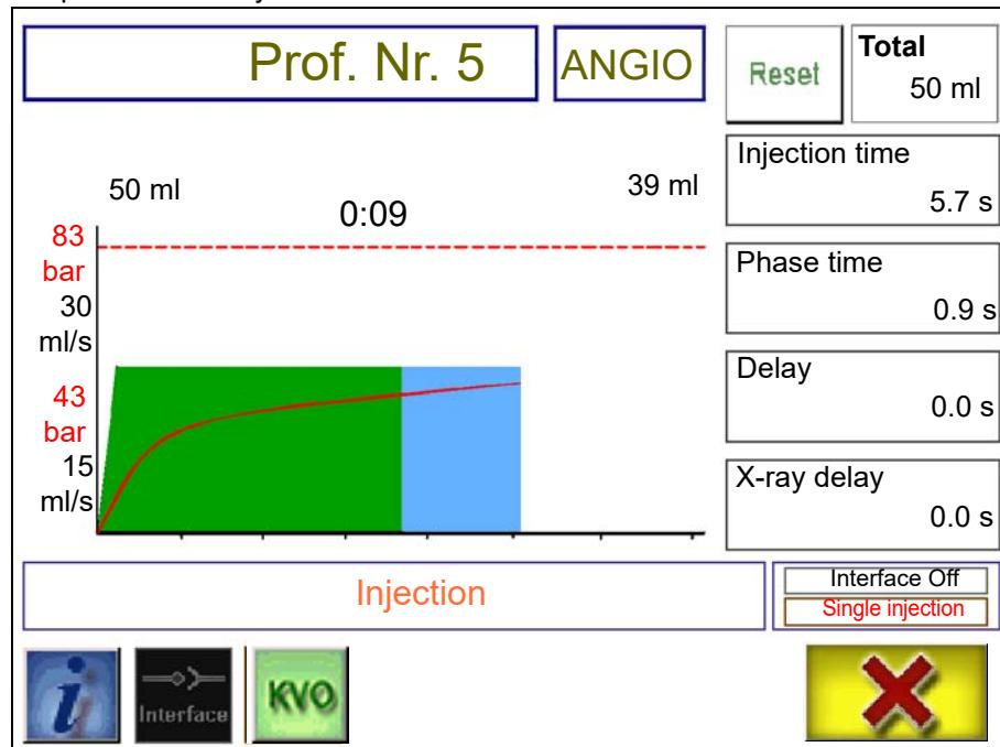
The flow rate is illustrated by the green field for contrast medium and by the blue field for NaCl and is running with the injection time.
