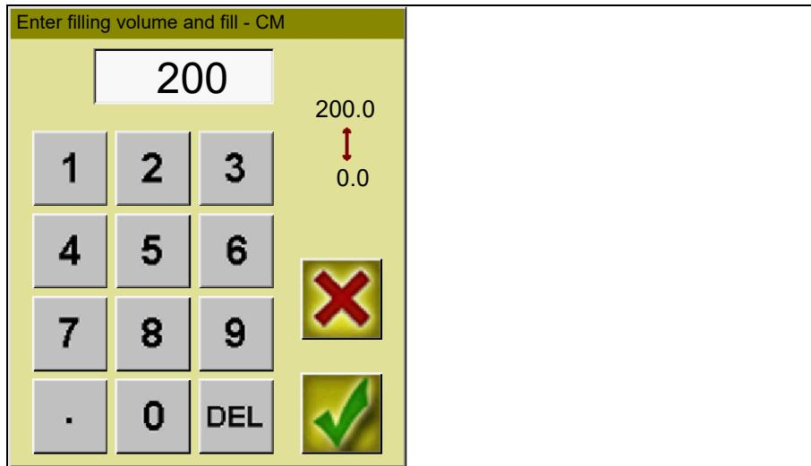
The range which you can enter, e.g. 0.0 – 200.0 (ml), is in the top right of the dialogue window **Enter filling volume and fill – CM**.
