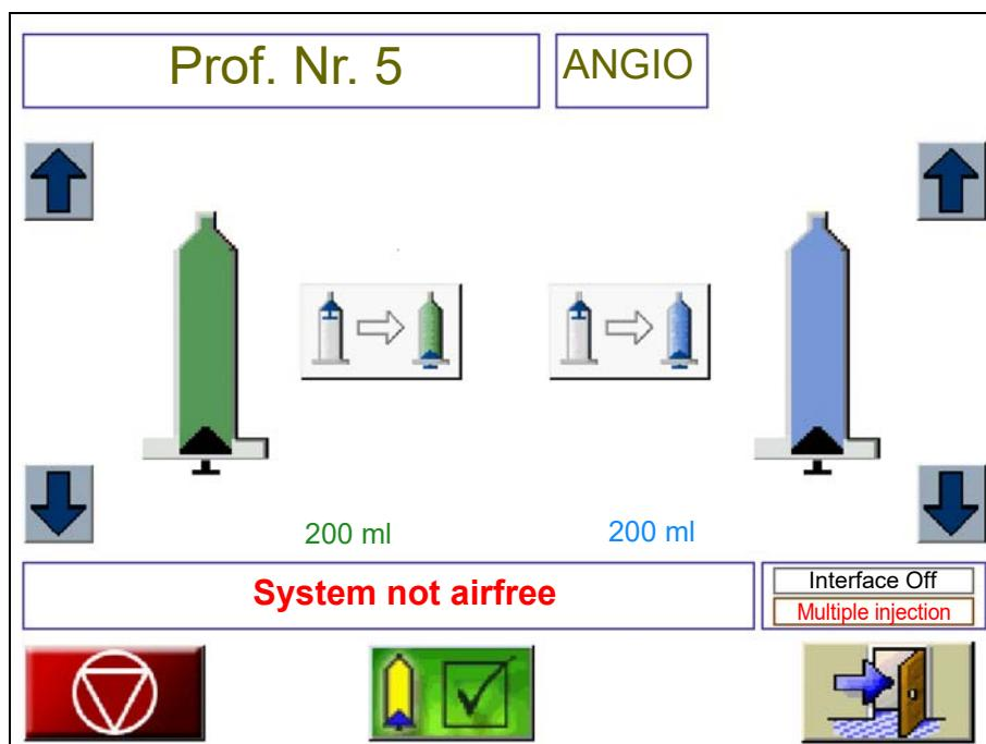
The piston is retracted when it is right at the bottom of the syringe, the syringe is completely green/blue and the remaining volume displayed is 200 ml (see diagram).
