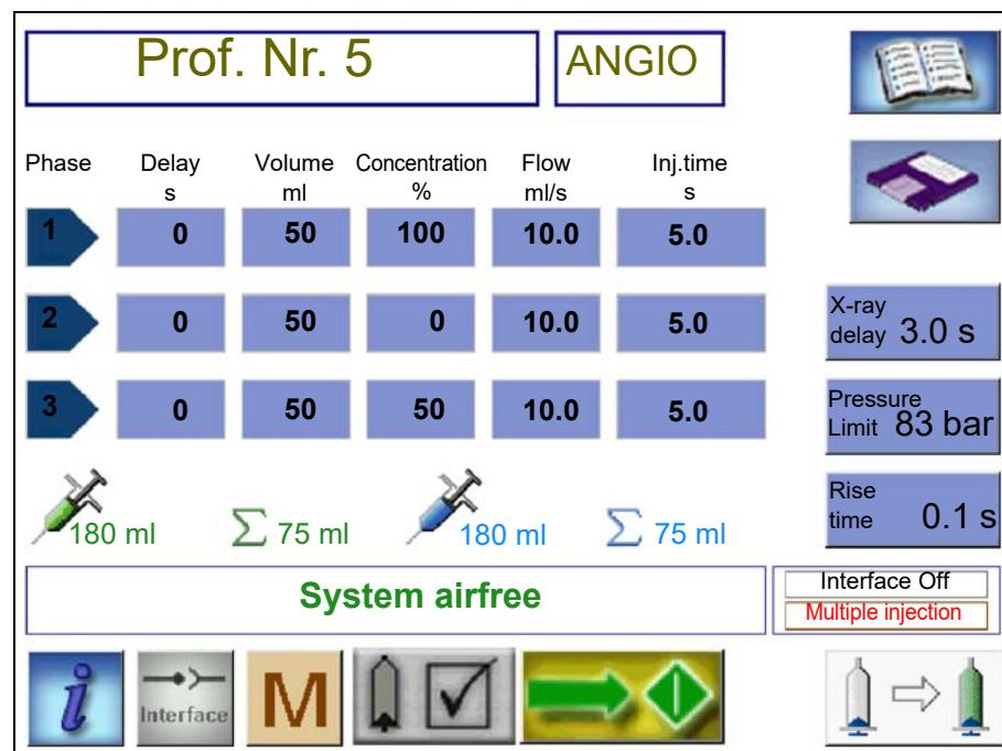
In addition to entering commands, the main window of the touch screen also serves to display the process information currently set. The profile name is located in the text field in the top and the parameters of the injection profile currently selected are in the table underneath.
