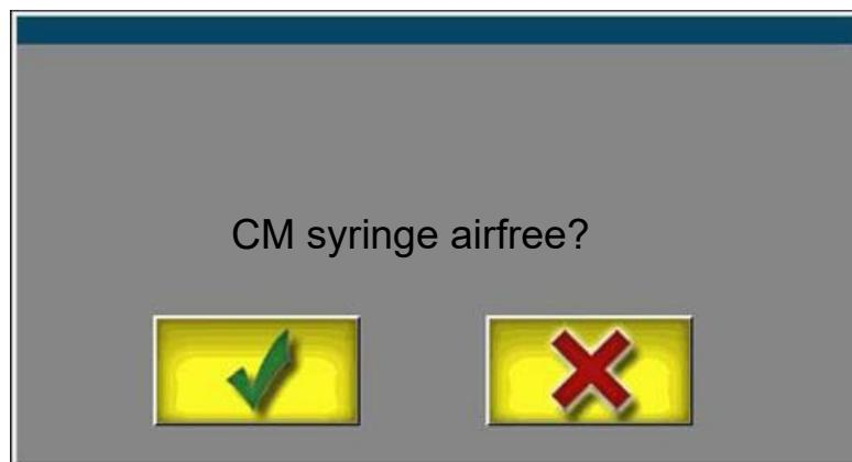
You answer dialogue messages by touching the relevant button. In the example shown above you can either confirm the question "CM syringe airfree?" by touching the button with the green symbol **Confirm** or negate the question by touching the button with the red cross **No/Reject**.
