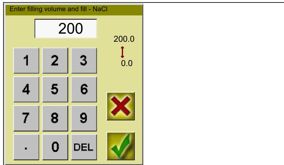
The range which you can enter, e.g. 0.0 – 200.0 (ml), is in the top right of the dialogue window **Enter filling volume and fill – NaCl**.
