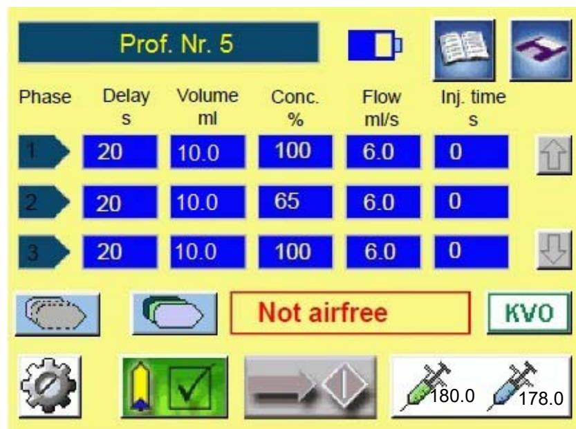
In addition to entering commands, the main window of the touch screen also serves to display the process information currently set. The profile name is located in the text field in the top left and the parameters of the injection profile currently selected are in the table underneath.
